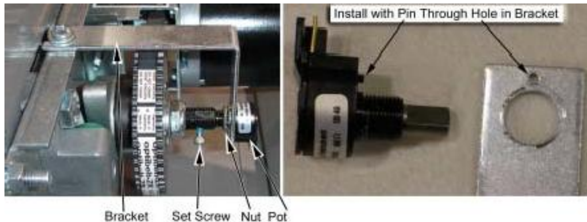
Figure 30. Replacing the 5 K \Omega Steering Pot
