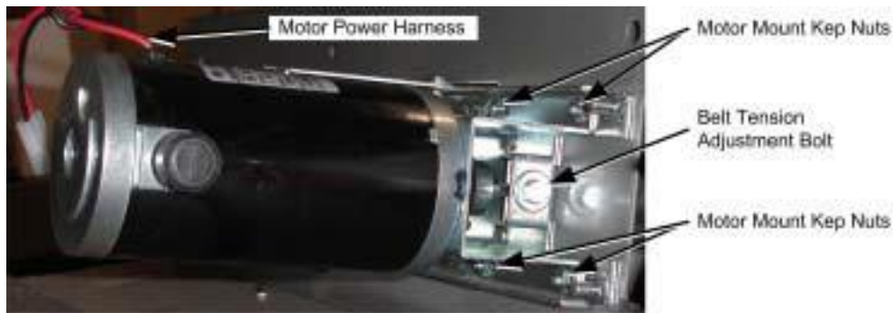
Figure 31. Servicing the Steering Motor
