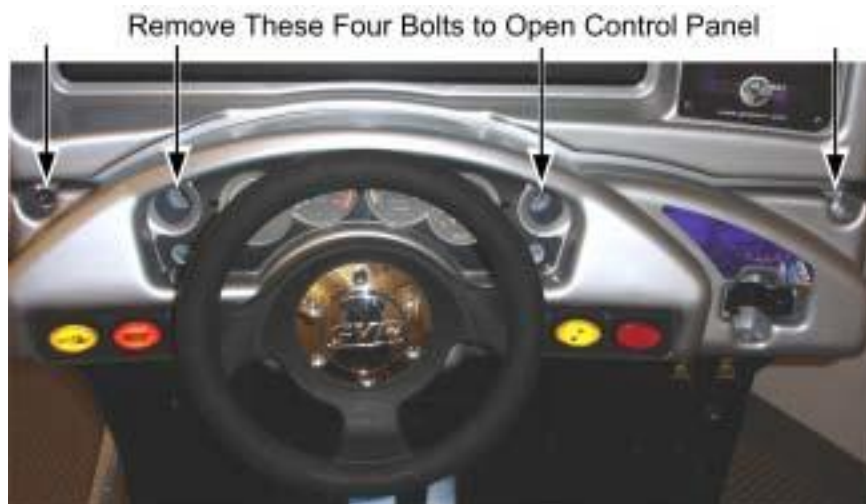
Figure 28. Opening the Control Panel
