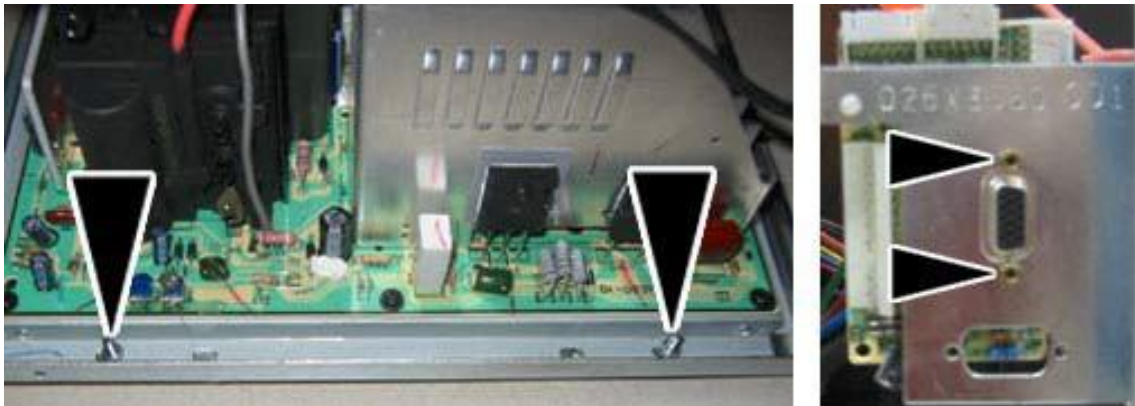
Figure 38. Removing the Monitor PCB Mounting Hardware
