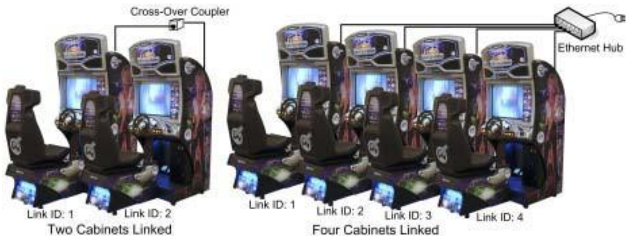
Figure 6. Linking Cabinets Without Broadband
